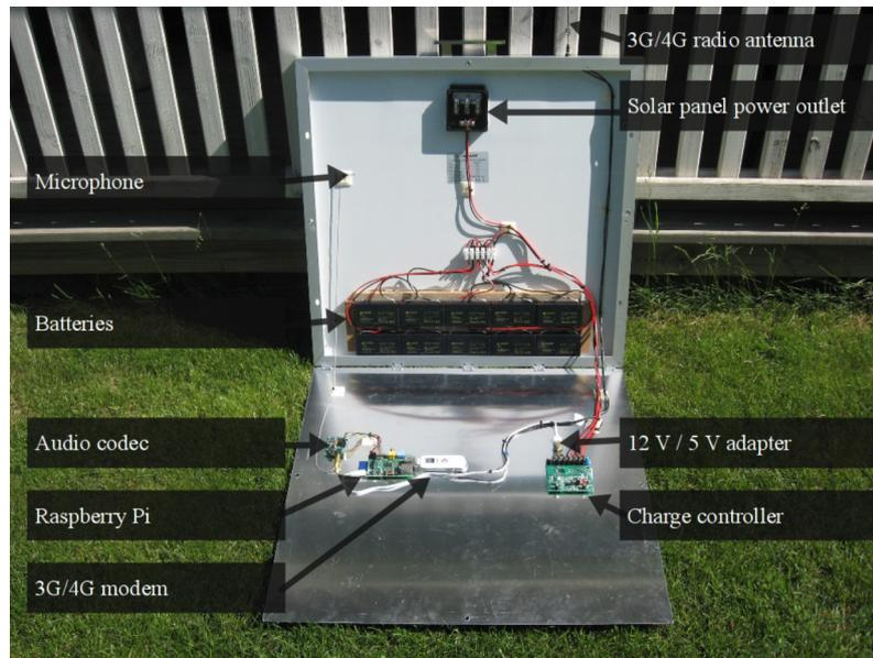
Fig. 2. A prototype version back cover opened.
