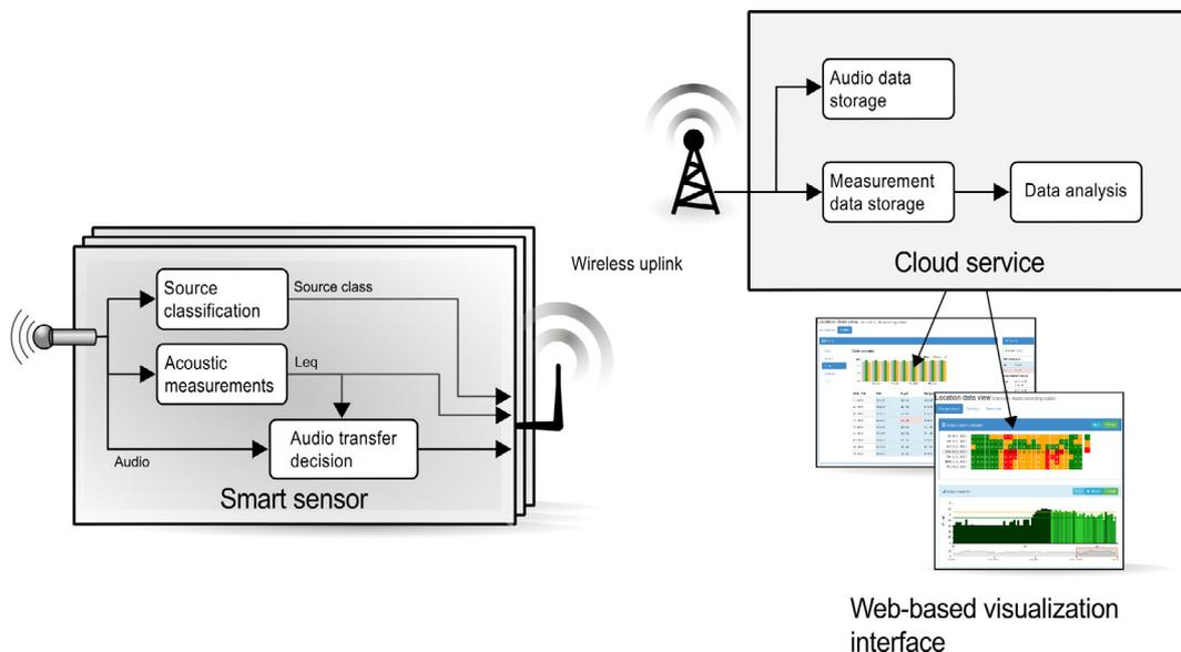
Fig. 1. Block diagram of the noise monitoring system.
