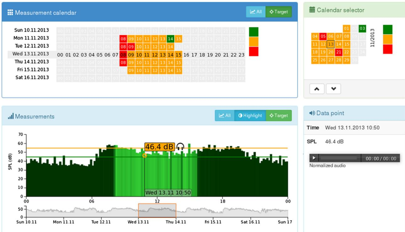
**Fig. 3.** Example view of the noise monitoring portal. In the upper right corner there is a calendar selector with day view. By selecting a day, more detailed data of the day is shown in a calendar view and in a graph view at left. The measurement calendar shows measurements assigned to the target source, and in the graph view target presence is shown with intensity of the colour. An audio playback is shown in the lower right corner.
